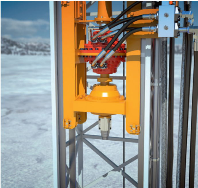
▲ Drilling /top drive
